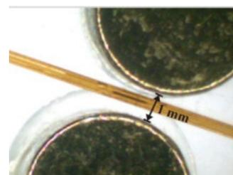
Sample preconcentration is done inside the capillary using anti-AGP antibodies magnetically fixed inside the capillary
